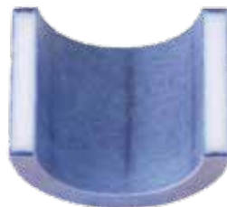
Comparative sample of a 99.7% \text{Al}_2\text{O}_3 ceramic; the cross-section clearly shows corrosive attacks of the microstructure.
