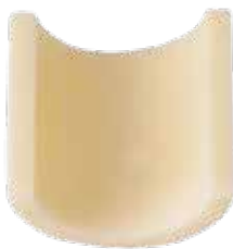
DEGUSIT AL23 sample after the corrosion test described below. The absence of methylene blue staining indicates that sulphuric acid did not corrode the microstructure.
