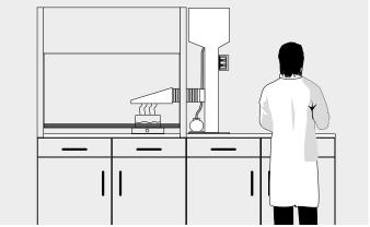
The fume scrubber C20 is flexible in its installation in the laboratory. Besides an installation on laboratory benches or on the floor it can be placed where the installation of a fixed scrubber is not possible due to restrictions of space. Please note that the unit must not be installed inside a fume cupboard.
